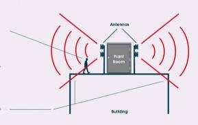
Each Scenario is indicative and a simplified version to demonstrate the technical constraints and solutions. Although 2D was used for simplicity, antennas must be carefully sited at locations on a building to provide 360 degree coverage, and must always be ICNIRP compliant.
